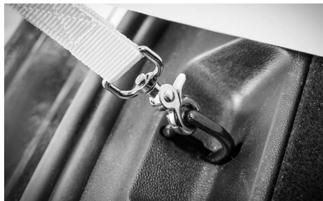
Figure 4 : Fixer le mousqueton
