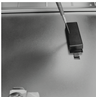
Figure 3: Opening the battery case lid
