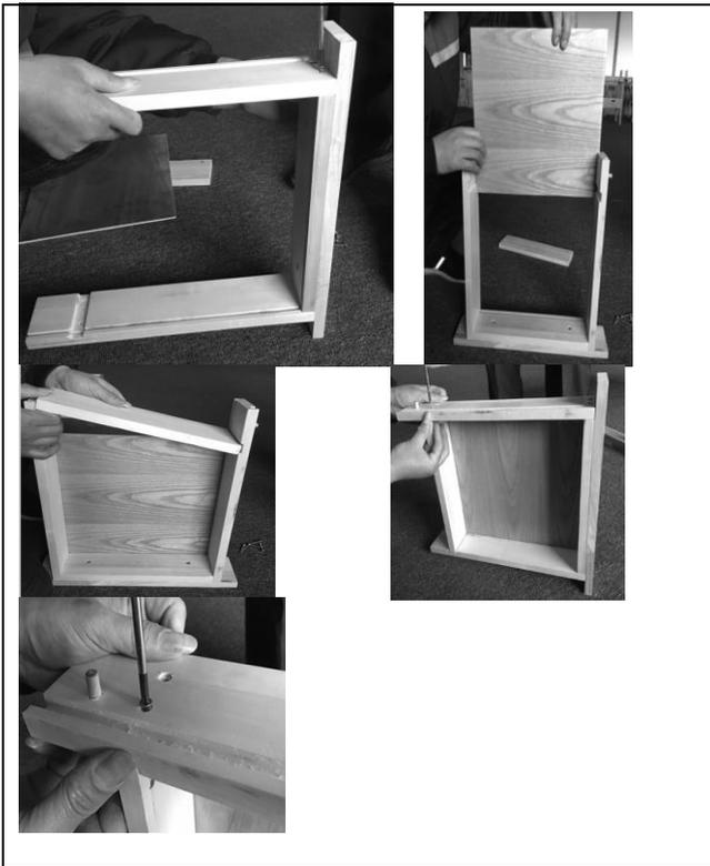
a. Assemble the components as shown and secure with screws.
