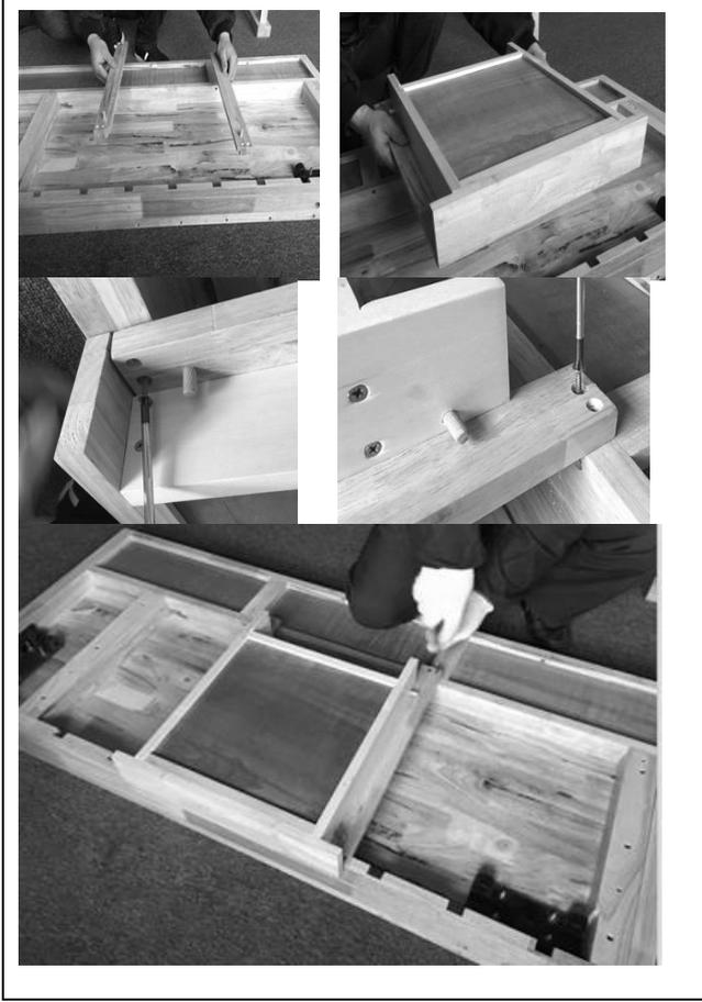
b. Fasten the two drawer runners with the groove in the drawer as shown.
