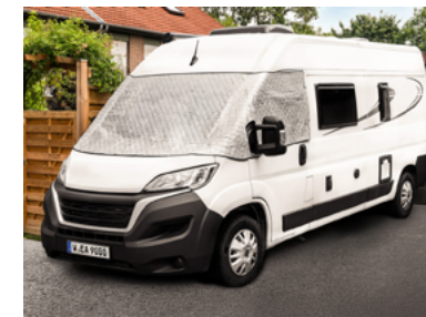
Image 3: Window protector fitted
