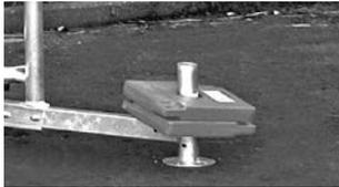
The picture shows a ballast element on the stabilizer.
