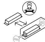
Light source (LED) is replaceable only by a professional.
