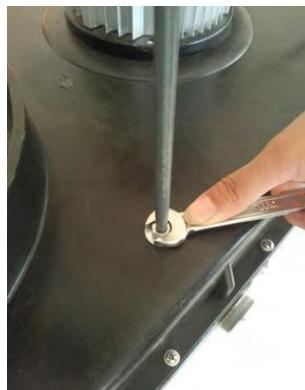
7. Set the bag on the fan wheel housing and tighten the bag clamp, then hang the filter bag on the bag support
