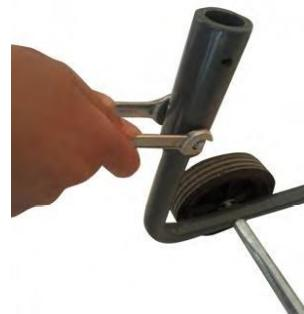
2. Set side bracket into the connector, use the bolt M6x35mm thread the hole and tighten them.
