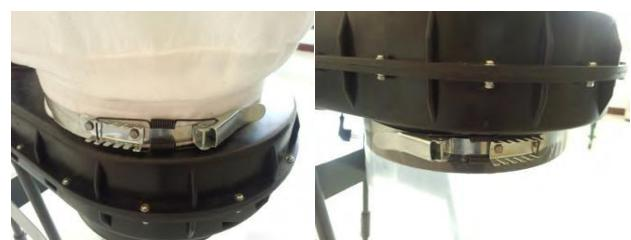
8. Set the hose on the fan wheel housing and tighten the hose clamp
