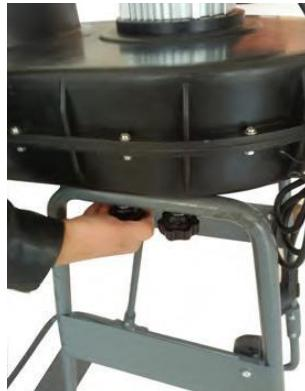
6. Install the bag support on the fan wheel housing.
