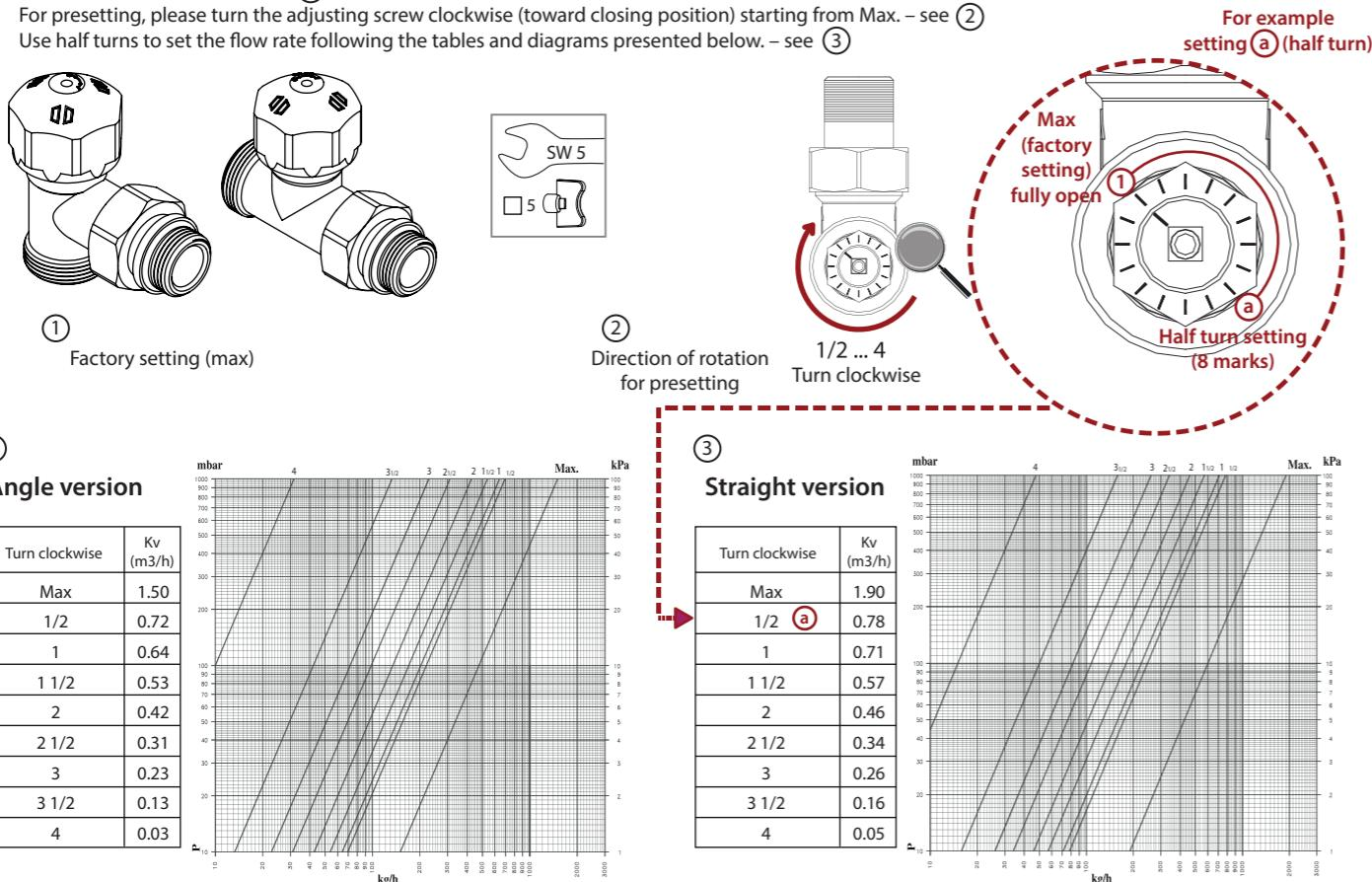
Max. Differential pressure = 0,04 – 0,2 bar (4 – 20 kPa, recommended 10 kPa)
