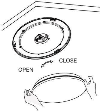
Put on the lamp cover and rotate it clockwise to fix.
