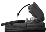
Figure 4: Closing the battery snap connector
