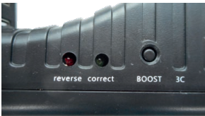
Figure 3: Start box control lights
