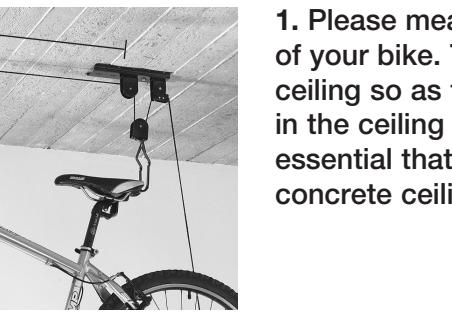
1. Please measure the distance between the handlebars and the saddle of your bike. This distance is the measurement you transfer to the ceiling so as to mount the base. For mounting, use a drill to drill holes in the ceiling and screw the base plate to the ceiling. Attention: it is essential that you use dowels for the ceiling holes when drilling into concrete ceilings, in order to ensure a secure hold.
