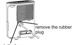
Attach the hose to the drain hose outlet.
