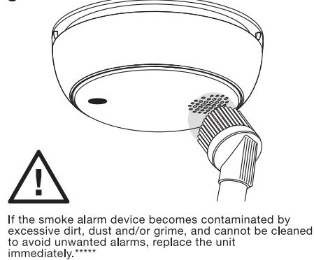
If the smoke alarm device becomes contaminated by excessive dirt, dust and/or grime, and cannot be cleaned to avoid unwanted alarms, replace the unit immediately.\*\*\*\*
