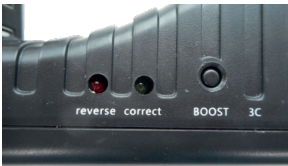
Figure 3: Start box control lights
